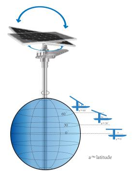
Light Post Installation Height Recommendation Diagram (Solar Sailing Light III)
