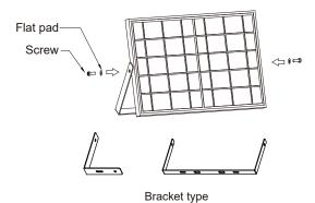
The bracket is agligned with the holes on both sides of solar panel, and fixed by screw and washer.
